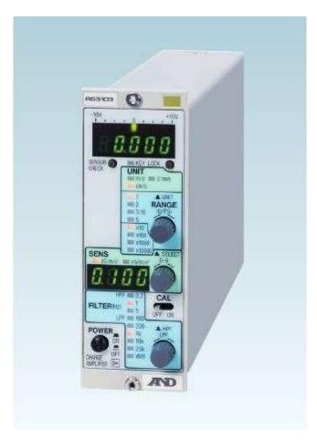
The AG3103 is our original charge amplifier that allows wideband (0.2Hz to 100kHz) signal input by floating the input / output and power supply system. The sensor is capable of multi-input, and by expanding the measurement range (~ 100,000m / s2) (10 times compared to the conventional one), it is possible to measure a wide range of vibrations from noise to impact.
