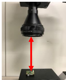
15 \mu\text{m} microscopic lens Focal distance: 195mm
