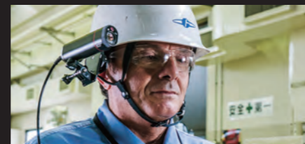
The camera-head can be attached to a helmet with a sense of wearable or the controller, and can be attached to a pole as camera stick.
