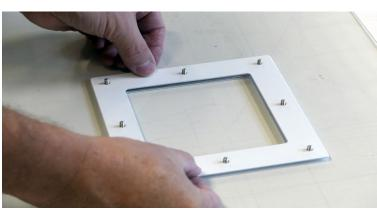
8. Replace the hex nuts or wing nut on the ClearIR-4-P by hand then tighten as needed with 5/16 socket or wrench.
