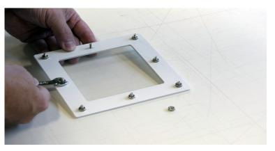
6. Place front plate with polyomer optic into cut out.
